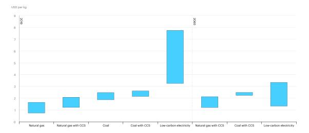
Source: IEA. (2019). *Global average cost of hydrogen production by energy source and technology, 2019 and 2050.* https://www.iea.org/data-and-statistics/charts/global-average-levelised-cost-of-hydrogen-production-by-energy-source-and-technology-2019-and-2050
