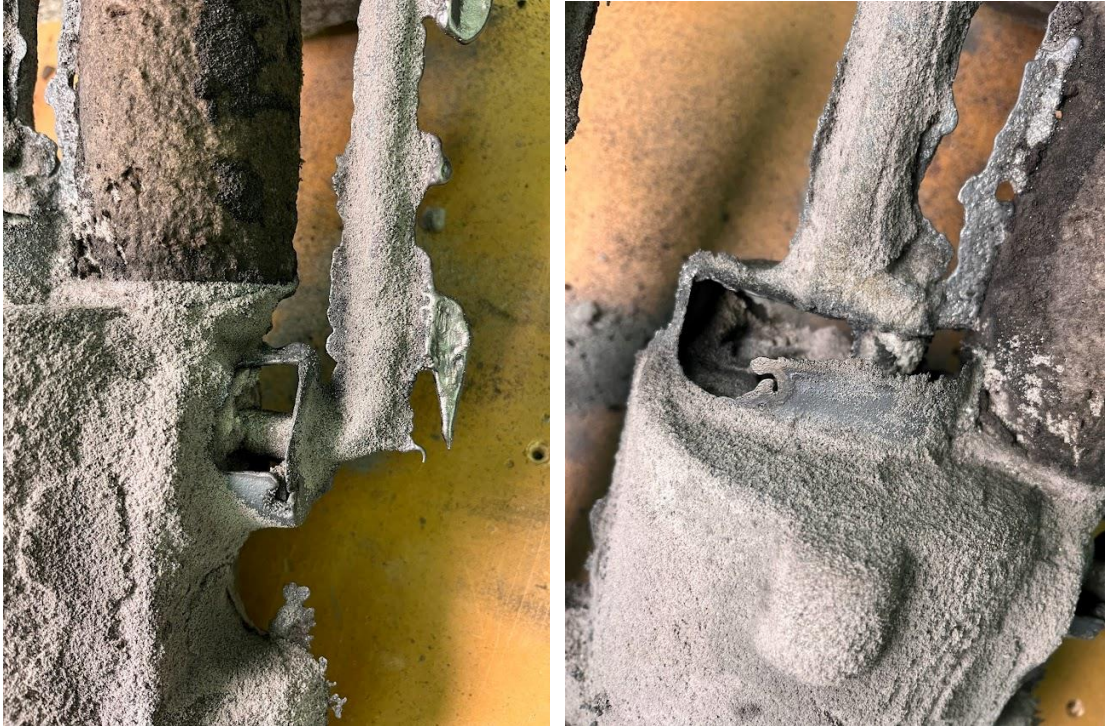
Figures 4-21 and 4-22: Severe flash around both the intake and exhaust core prints. This caused the air vents to fill up, preventing VOCs from escaping.
