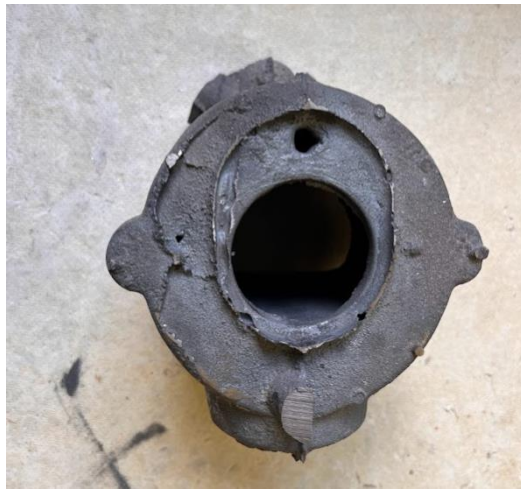
Figures 4-14 and 4-15: Results from the fifth attempt at the manifold pour. There were two small holes on the top, resulting from not enough material left over after the significant bulge in the right picture.
