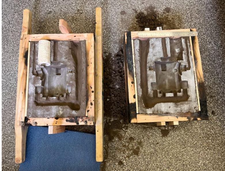
Figure 4-28: Second attempt flask layout.
