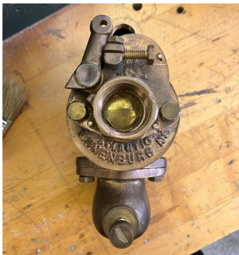
Figures 4-4 and 4-5: Original carburetor made in Lunenburg and a diagram explaining the Venturi principle that mixes the air and gasoline.
