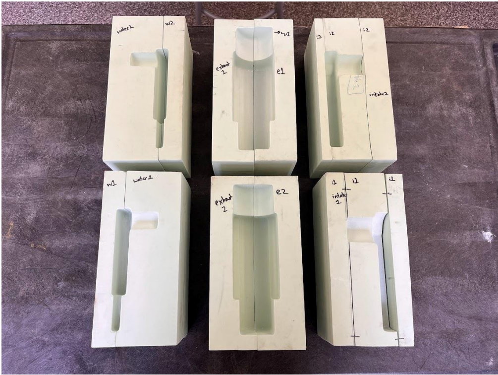
Figure 4-27: New core boxes, two for each core because each is made in two halves and then glued together.
