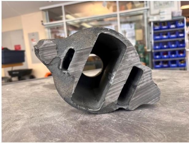
Figure 4-29 and 4-30: Second attempt results, showing solid walls and uniform wall roughness.
