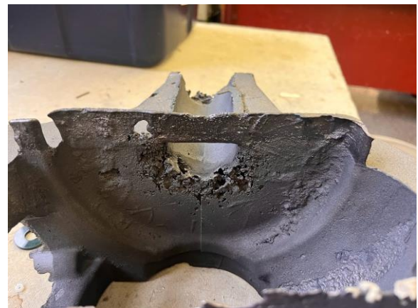
Figures 3-4 and 3-5: Poured part by Liang in 2019, one end has defects due to sand that was trapped in the iron's way, requiring a part redo. You can see the gate along the center line in the picture to the left.
