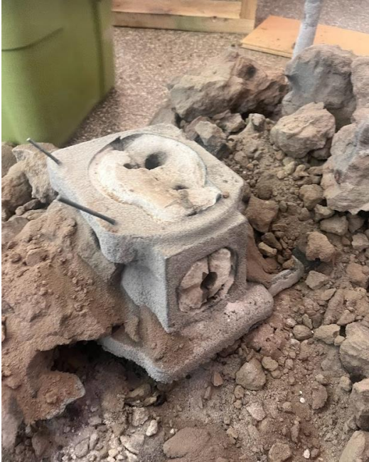
Figures 3-19 and 3-20: Pouring molten iron into the flask, breaking the part out of the flask the day after the pour, looks good so far!
