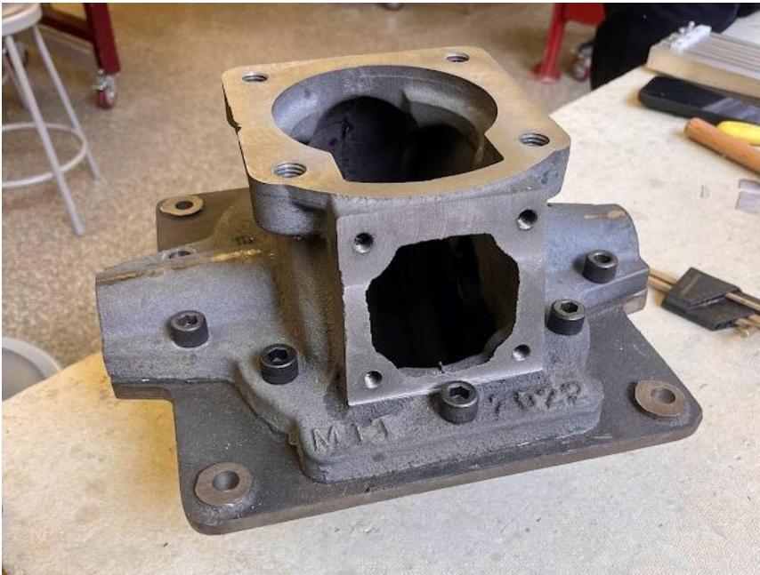
Figure 3-26: Finished upper base bolted to the lower base.
