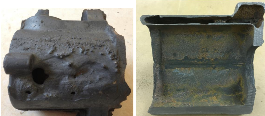
Figure 4-7 and 4-8: Various defects from the second and third pour attempts, suggesting a vertical orientation would likely work better.
