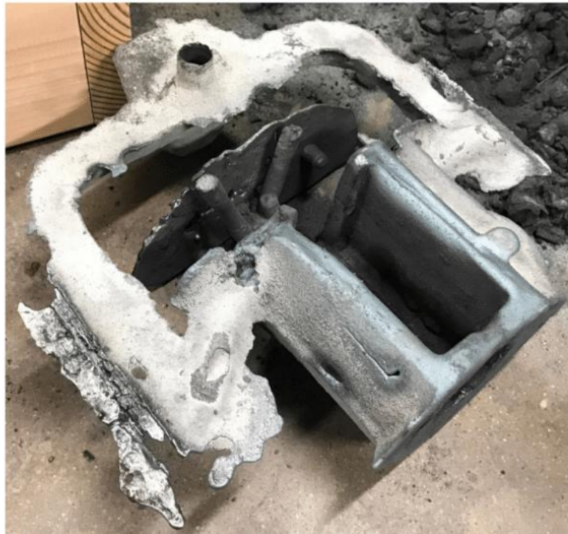
Figure 4-10: Fourth attempt at casting the manifold, resulting in a short shot due to significant core flash.
