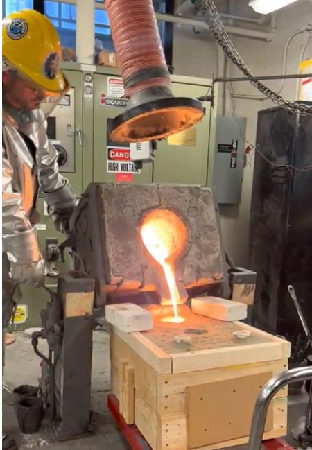
Figures 3-19 and 3-20: Pouring molten iron into the flask, breaking the part out of the flask the day after the pour, looks good so far!
