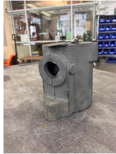
Figure 4-29 and 4-30: Second attempt results, showing solid walls and uniform wall roughness.
