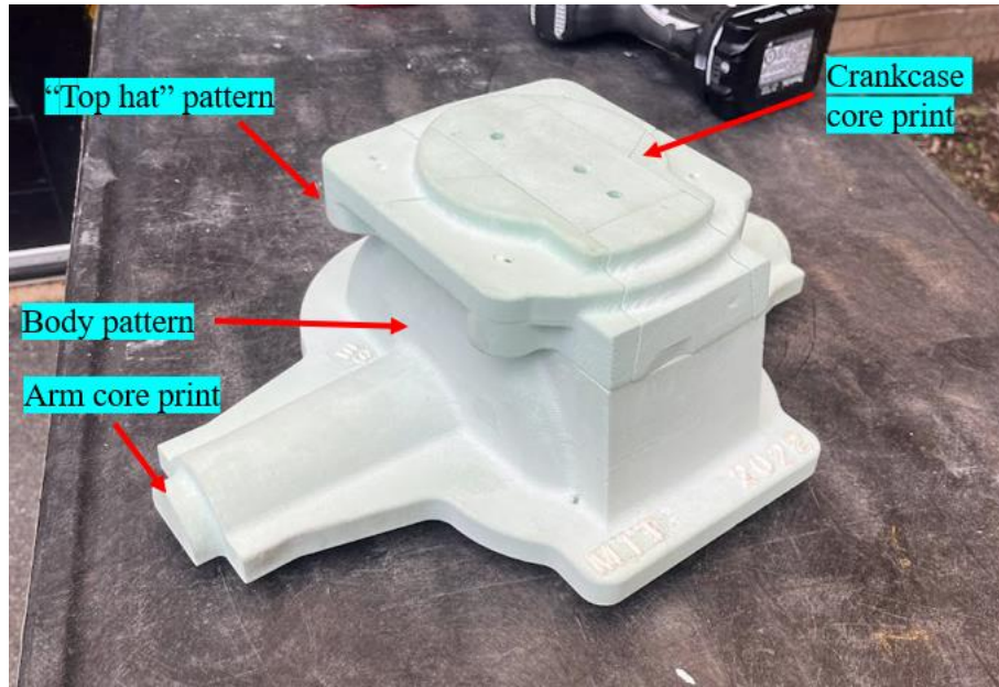
Figure 3-7: Machined upper base pattern, showing the two main sections and the core prints on the “arms” and crank case.
