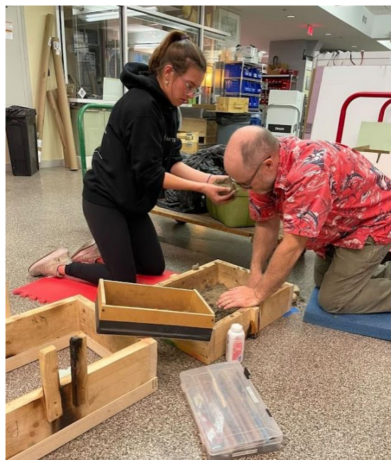
Figure 3-14: Packing the flask, parting line on the floor.
