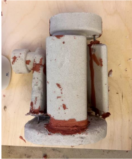
Figure 4-17: Mushy core puck and broken core.
