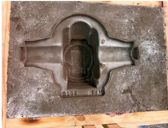
Figure 3-17: All pattern sections removed, you can see the “MIT 2022” and my initials imprinted into the sand.
