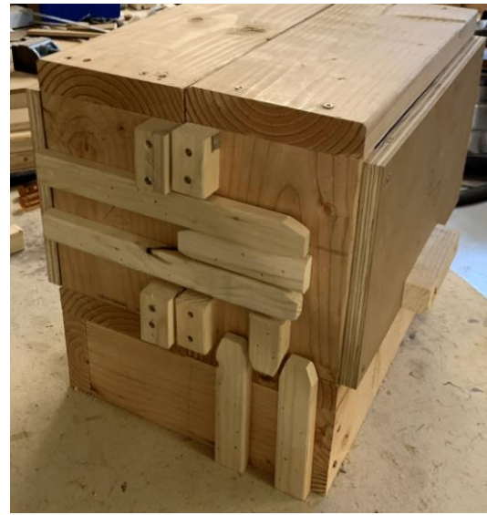
Figures 4-12 and 4-13: Vertical pour orientation and 3-part flask set up, Chiaki Kirby, Spring 2020.
