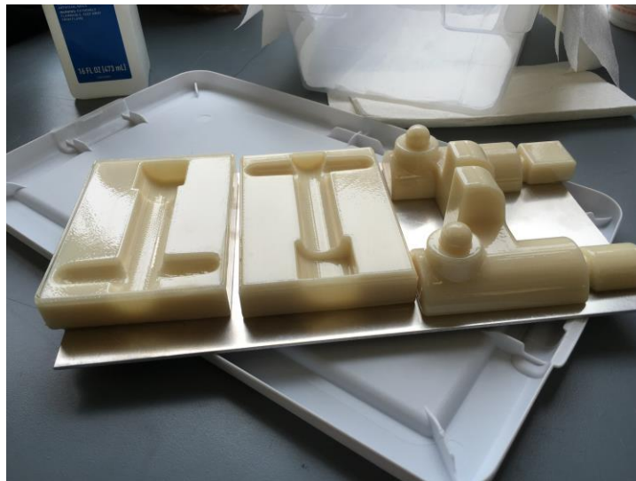
Figure 2-7: Core boxes and patterns of the water pump from 2016.
