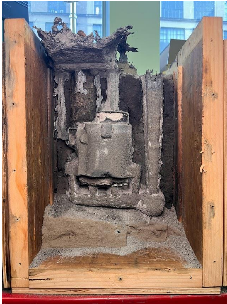
Figure 4-20: Cast part, dug out along the parting line to see the path the iron took as it filled the part. The iron contacted the wood on the left side of the flask, causing the wood around the parting plane to catch on fire.
