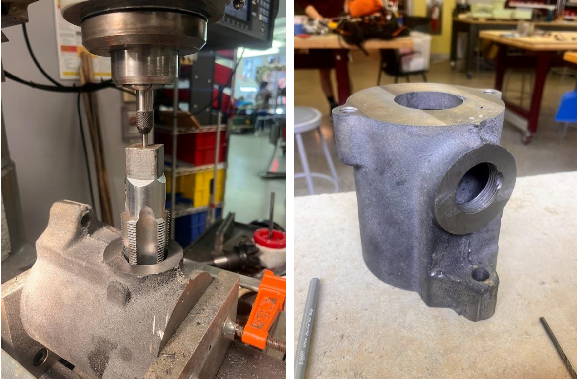
Figure 4-35 and 4-36: Tapping the carburetor hole and the completed part!
