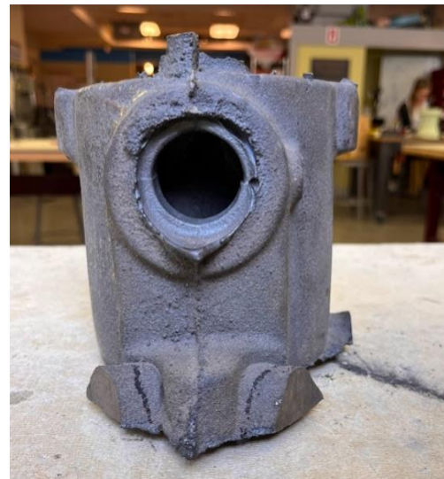
Figures 4-14 and 4-15: Results from the fifth attempt at the manifold pour. There were two small holes on the top, resulting from not enough material left over after the significant bulge in the right picture.
