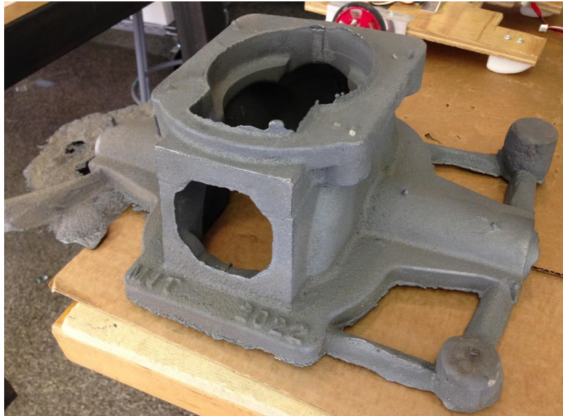
Figure 3-21: Poured part with risers, gates, and well still attached. Minor flash around core prints.
