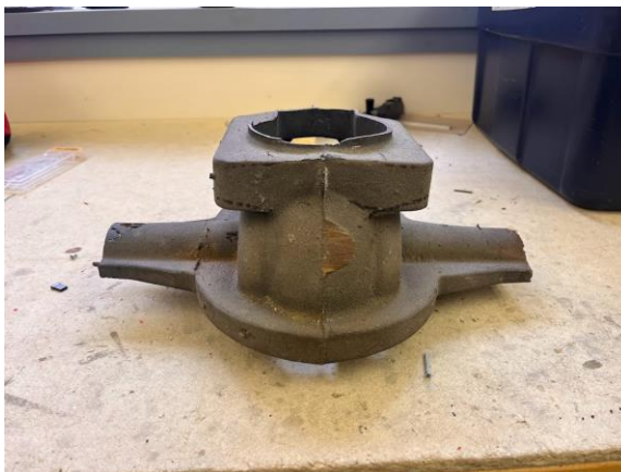
Figures 3-4 and 3-5: Poured part by Liang in 2019, one end has defects due to sand that was trapped in the iron's way, requiring a part redo. You can see the gate along the center line in the picture to the left.
