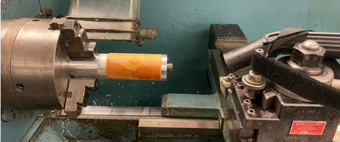
Figure A-1: A tool was made for mounting the liner pieces to a lathe for turning down the outer diameter.
