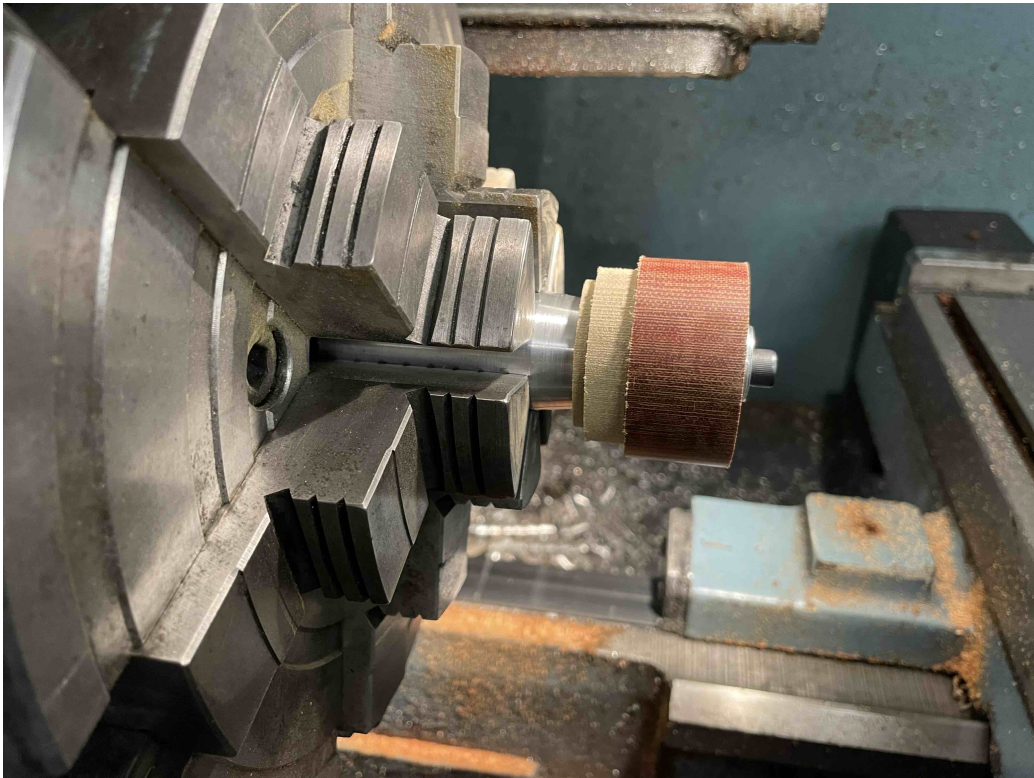
Figure A-3: A custom tool was developed for mounting the aft insulator to the lathe for machining the external geometry.
