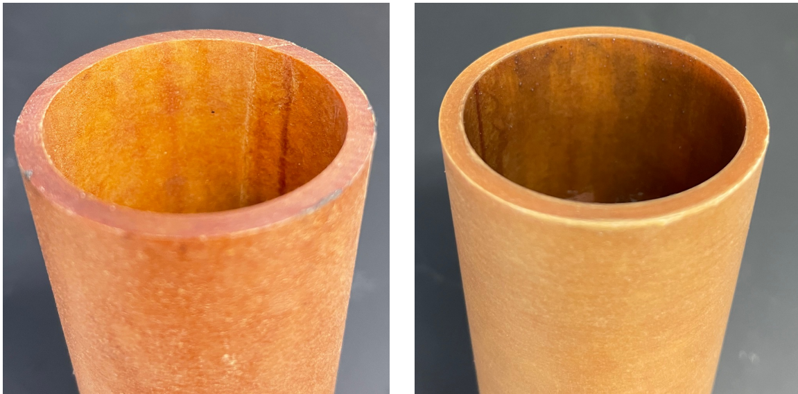
Figure A-2: A primer is applied to the inner surface of the propellant insulator to promote good bonding between the insulator and the propellant. Left subfigure: unprimed insulator. Right subfigure: primed insulator.
