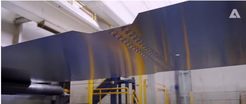
FIGURE 9: MECHANICAL STITCH PHYSICALLY CONNECTING TWO SEPARATE COILS IN THE CCL PROCESS (ANDRITZ)
