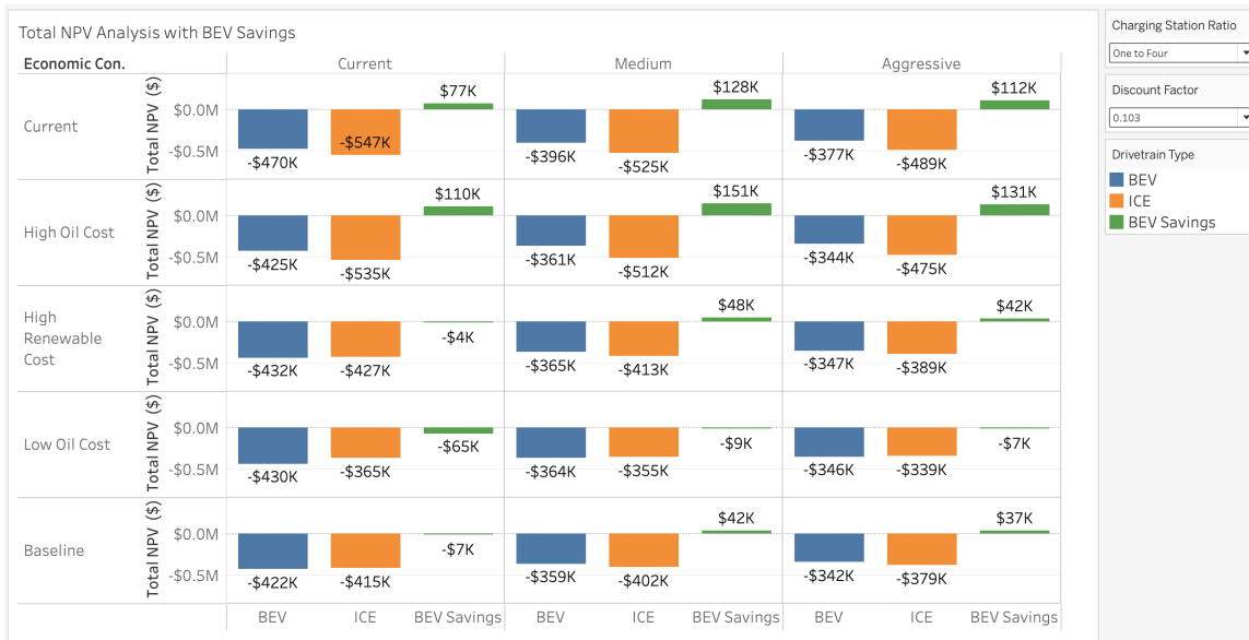
Figure 6-10: Total NPV Analysis with BEV Savings at the end of Expected Years of Ownership at 10.3% Discount Factor and Four-to-One Charging Ratio
