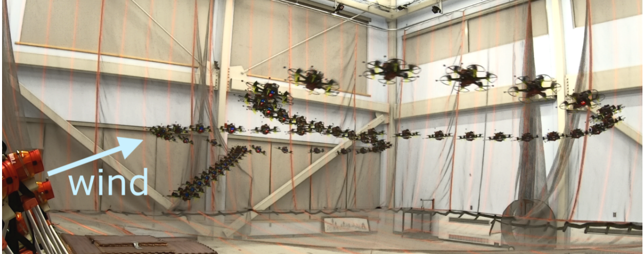
(a) Time-lapse of an experiment showing the trajectory executed by the robot, and the leaf blowers used to generate disturbances
