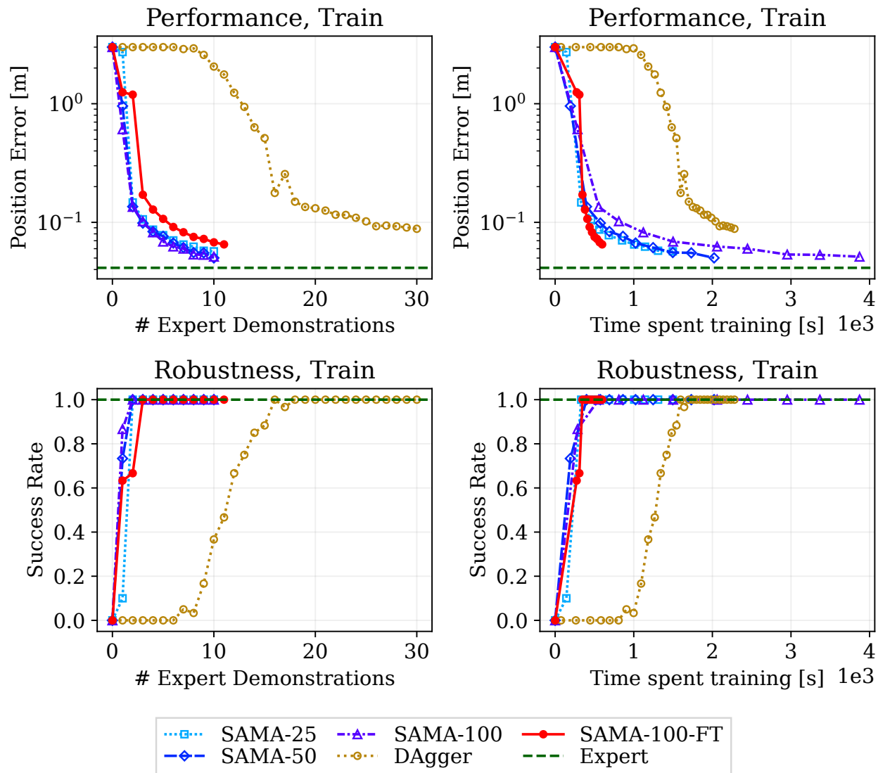
Figure 6.3: Performance and robustness in the training environment after Phase 1 , as a function of number of demonstrations and training time. IL allows for the learning of effective Phase 1 policies in one hour on a single core, as opposed to RL which has been reported to take two hours on an entire desktop machine [44]. This training time can be significantly shortened by using tube-guided data augmentation during training.
