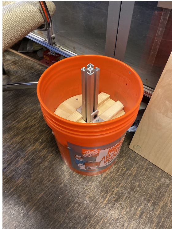
(b) Fully assembled buoy with 80/20 extrusion
