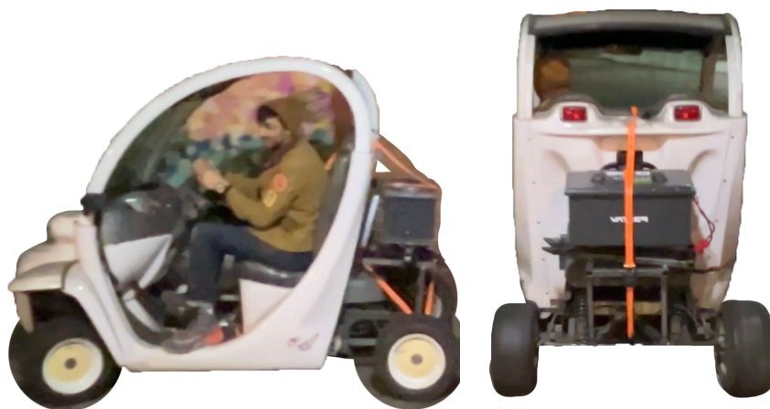
Figure 4.2: Above, the modified GEM with ball-groove KC's acting as physical and electrical connections is shown in operation. The battery is on the welded frame at the back of the vehicle. An orange ratchet strap applies preload to the system.
