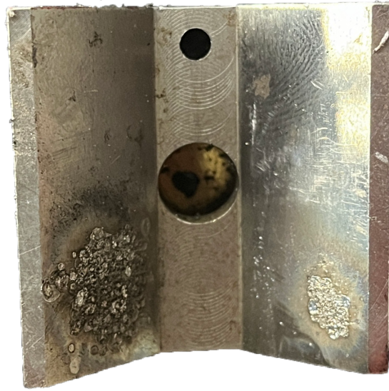
Figure 4.3: One of the KC's from the operated frame is shown above with the damage caused by arcing. Arcing occurred during vehicle operation because an insufficient preload allowed the couplings to separate as the vehicle drove over road irregularities.
