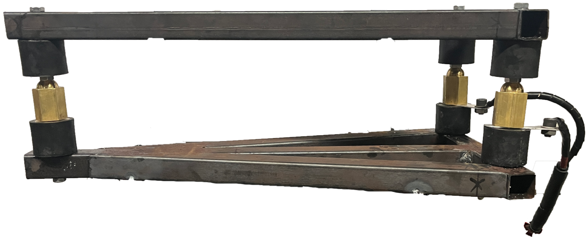
Figure 4.4: The finished damper ball and socket assembly is pictured above, with a flat plate of 1/16" thick aluminum ( R \leq 0.005\Omega ) used to complete the electrical connections from the sockets to the GEM. The battery is not pictured for clarity, but would rest on top of the assembly and similarly use aluminum to create an electrical connection with the KC balls.
