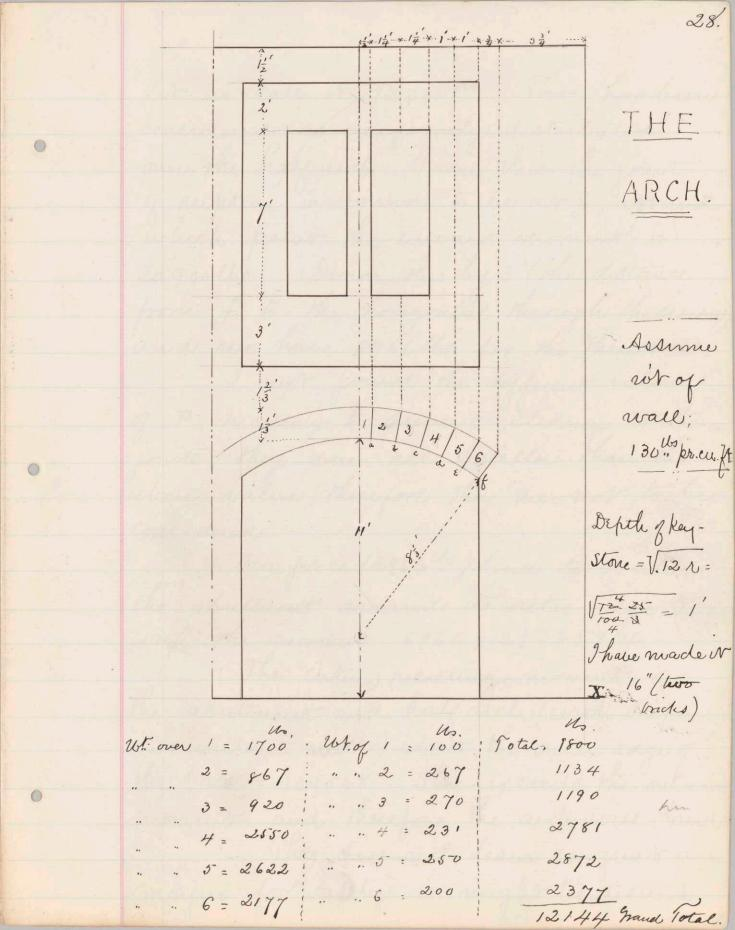
Let us call it 12000 ths. This has been considered as uniformly distributed over the half-arch. From this the joint I respective is found to be arf, around which point the invaid moment is 20 900 lbs. Divide this by 3 ( the distance from f to the horizontal through the crown) and we have 6966 lbs for the thrust I. I meet found the different values of P necessary to prevent sliding at the joints; they were all smaller than the above value, therefore they are not to be Considered.
