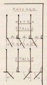
ENGINE ROOM. The extra stall have been placed directly behind the others, leaving a passage sufficiently large for cleaning operations. When the stall-doors a, a, a, open they close up the passage and allow the horses in the rear to pass out through the forward stalls. By this
