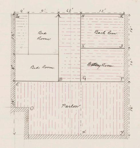
[Dotted red lines indicate the direction of the floor-jaists.] [all doors etc., have been omitted in the calculations and on the diagram.]
