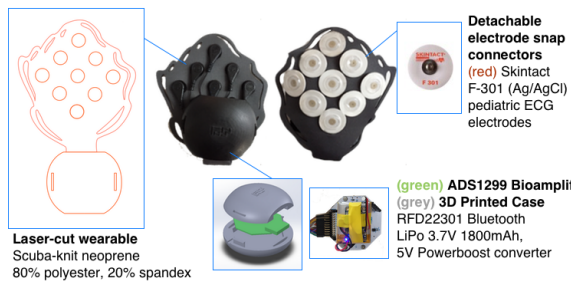
Figure 3: Wearable components. Includes laser-cut scuba knit neoprene, 3D printed case with bioamplifier, LiPo battery, and powerboost converter.
