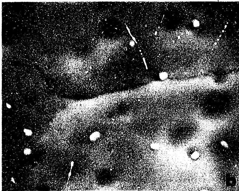
Figure 9 : Scanning electron micrograph of the chemically etched surface of annealed zircaloy 2. a) Low magnification view. b) Chromium rich particles.
