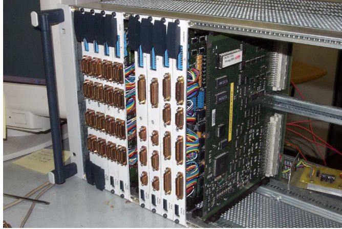
Figure 5-3: The engineering electronics crate. From the left to the right, 4 UGFV, 2 UGBC, 2 UGBS and 1 USCM cards. The engineering USCM does not have a front panel connector.
