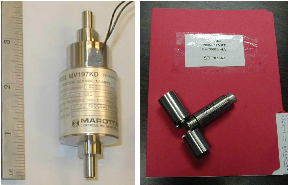
Figure 4-13: a) A Marotta MV197 valve. b) A GP:50 pressure sensor in a high pressure holder.
