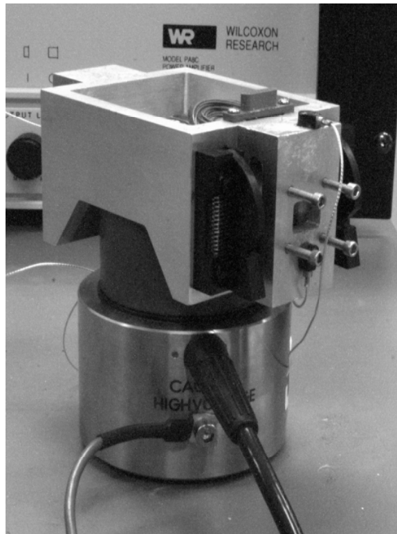
Figure 3-5: Photograph of Wilcoxon Shaker with Fixturing
