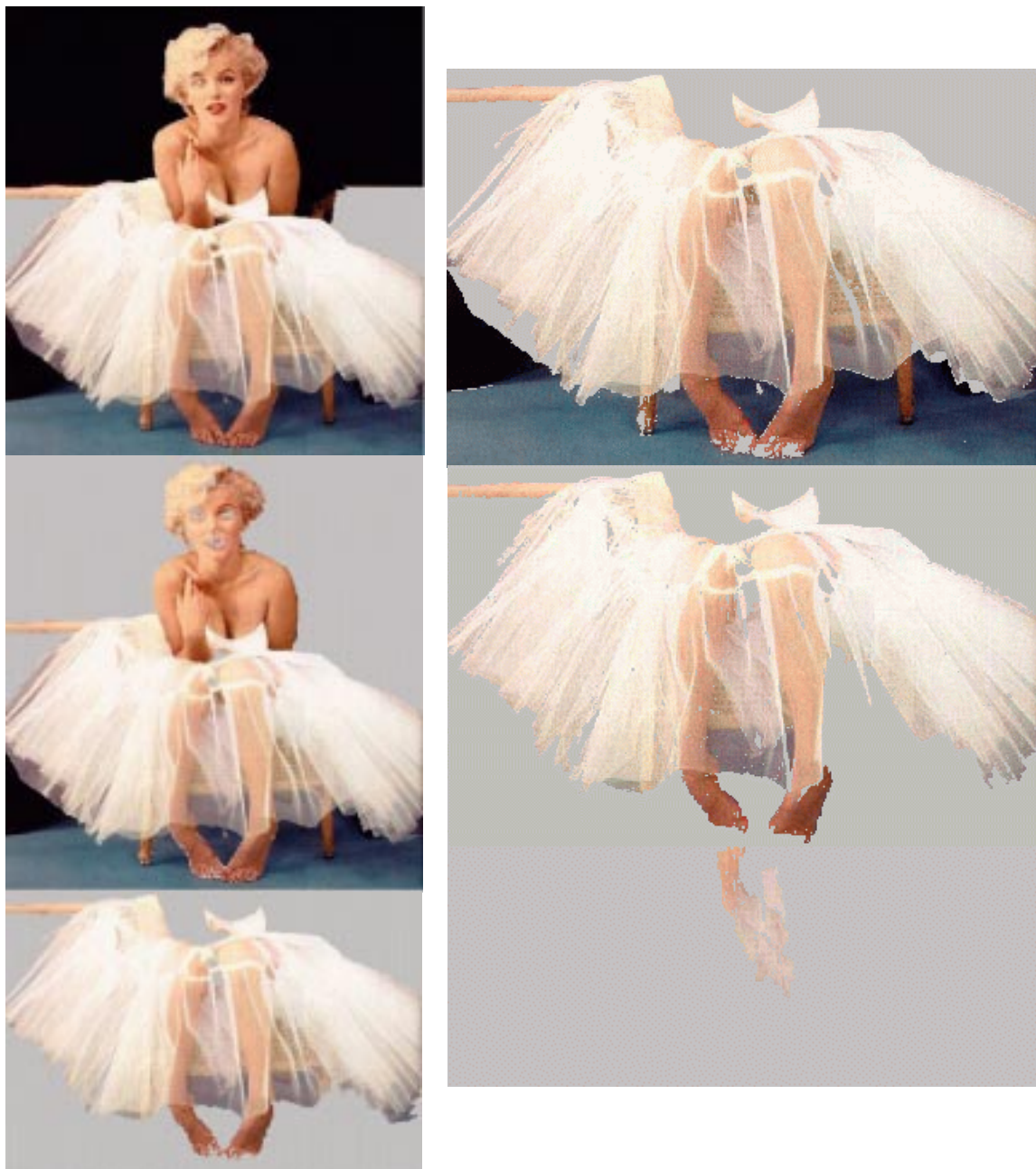
Figure 6-5: The performance of the Progressive Grow Algorithm using HSV color similarity on the left, and RGB color similarity on the right. The new pixel weighting for averaging is one fourth in both cases. The cutoff values from top to bottom for the HSV similarity are 0.84, 0.90 and 0.94, and for the RGB similarity are 0.76, 0.84 and 0.90.
