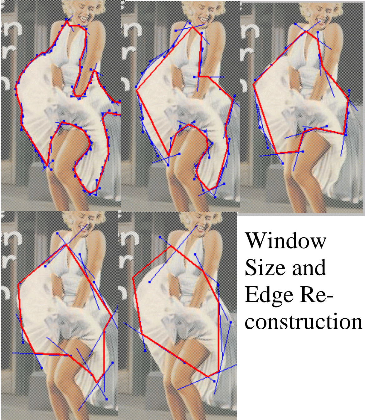
Figure 7-6: Decreasing the level of detail. A higher window size causes a greater tolerance to noise, and provides a rough estimate of the shape. A smaller window size allows more attention to detail, but also generates lengthier representations that might be harder to work with and might be overfitting noise from the segmentation.
