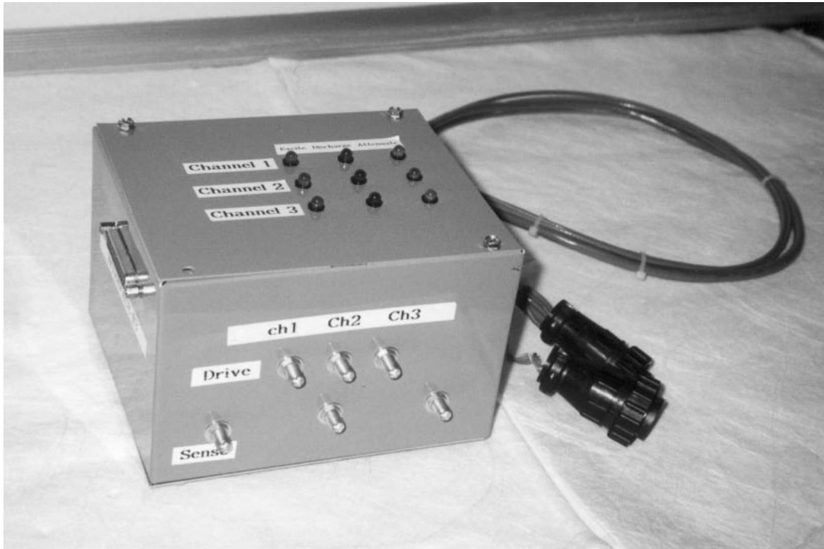
Figure 6.2: The new short-circuit interface box with the cable to the controller box connected at the back.
