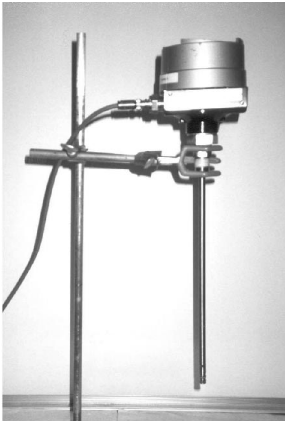
Figure 3.13: Harley CT-800 moisture sensor. The sensing element is at the bottom of the long rod.
