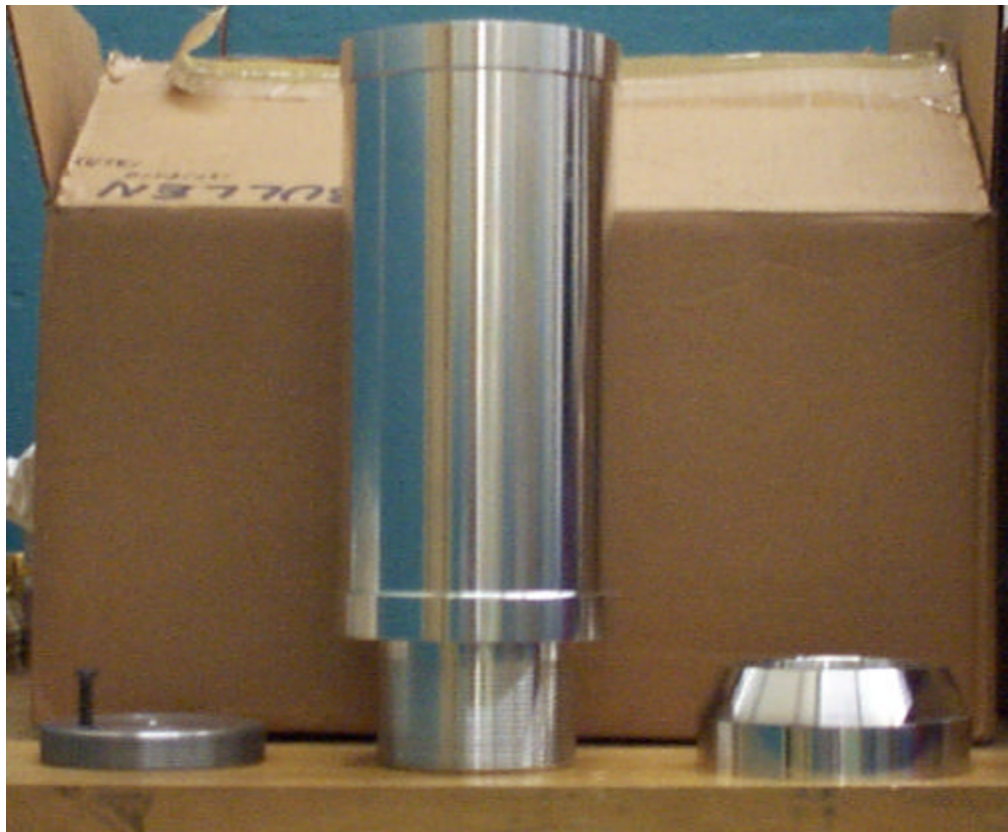
Figure 5.11: Custom machined canisters for air-gun tests
