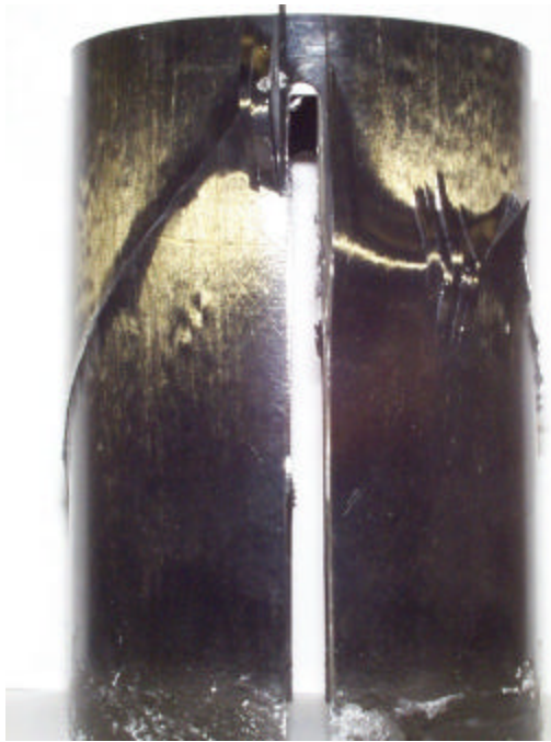
Figure 6.9: Buckled long slotted specimen
