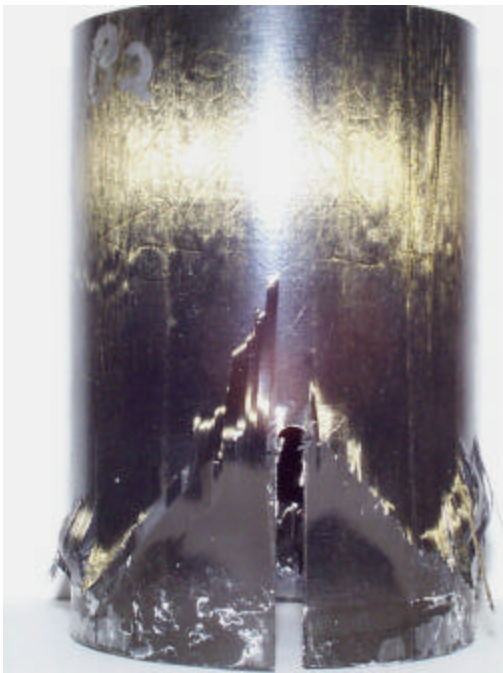
Figure 6.8: Fractured short slotted specimen
