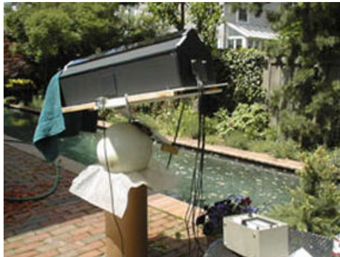
FIGURE B.1 TILTING MODEL AND MULTIPOSITION METER WITH SENSORS
