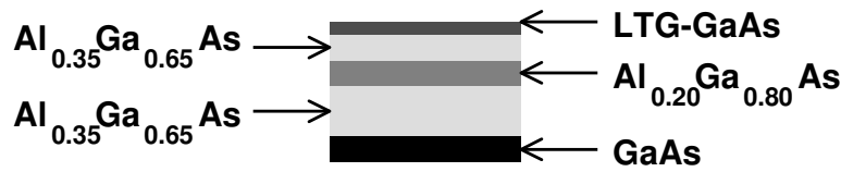
Figure 3-5: Schematic of the distributed photomixer epitaxial layer structure.
