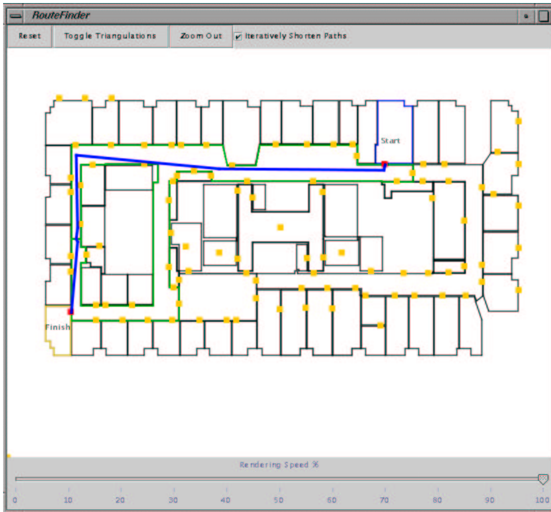
Figure A-1: The RouteFinder GUI. Users can view a map of a single floor, perform route finding, and test the results of different path filtering algorithms.
