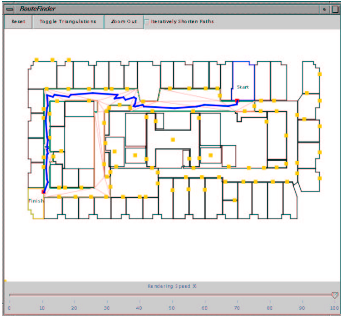
Figure 3-3: RouteFinder plots the same route as in Figure 3-1, but shows the triangulation in intermediate Spaces.
