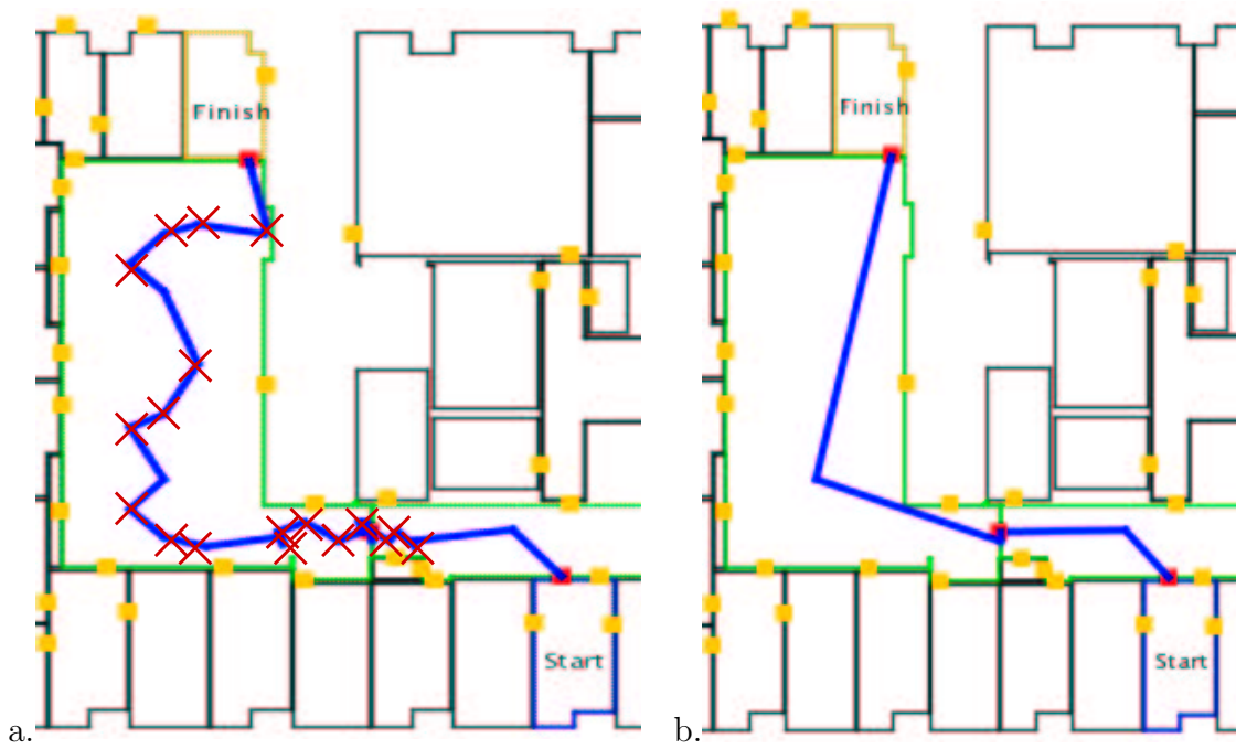
Figure 2-14: A path (a) is iteratively shortened, resulting in (b). Endpoints marked with an 'X' are eliminated, and their adjoining line segments condensed into a single segment.
