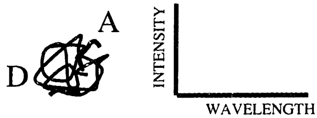
Figure 4-3: Intramolecular fluorescence quenching demonstrating quenching of donor dye when dye pair are within Förster distance.
