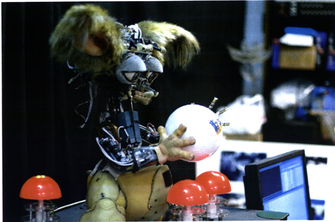
Figure 2-2: A photo of Leonardo, the emotionally expressive robot, holding a ball, and surrounded by some of the buttons he uses in object manipulation tasks.
