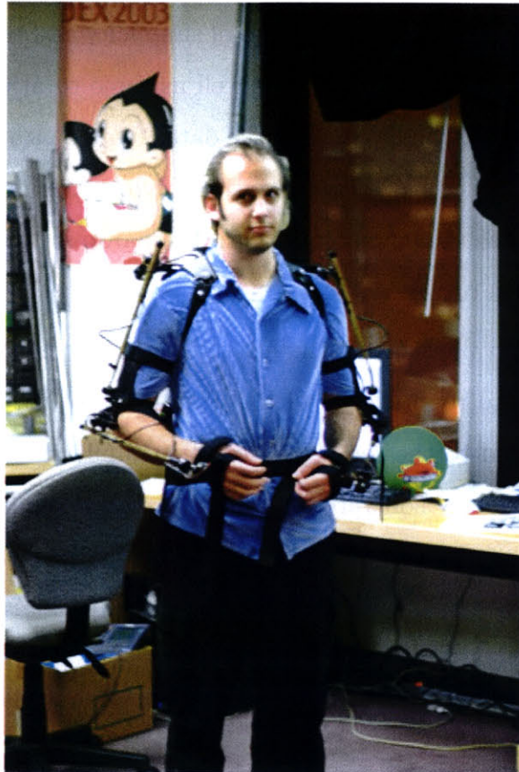
Figure 2-3: A Picture of the author wearing the Animazoo Gypsy Suit, a motion capture device used to collect motion data from a human participant as they perform some object oriented task.
