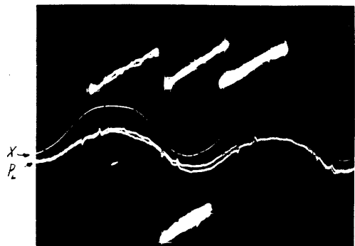
FIG. 2.8c Induced flow P_s = 1240 \text{ psig} , P_e = 220 \text{ psig} , \bar{P}_e = 455 \text{ psig} \bar{Q}_s = 1.35 \text{ gpm} , \bar{Q}_e = 2.2 \text{ gpm} , lower 200cps middle 200cps, upper left 20cps upper center 50cps, upper right 100cps
