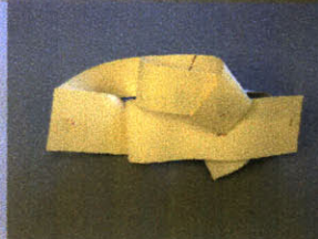
Min. Radius: 3" Forming: cold Properties: surface & structural along laminated axis
