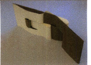
Min. Radius: 3" Forming: cold Properties: surface
