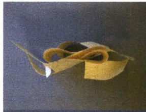
Min. Radius: 3" Forming: cold Properties: surface & structural along laminated axis
