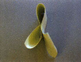
Min. Radius: 1" - 3" Forming: cold or hot Properties: surface
