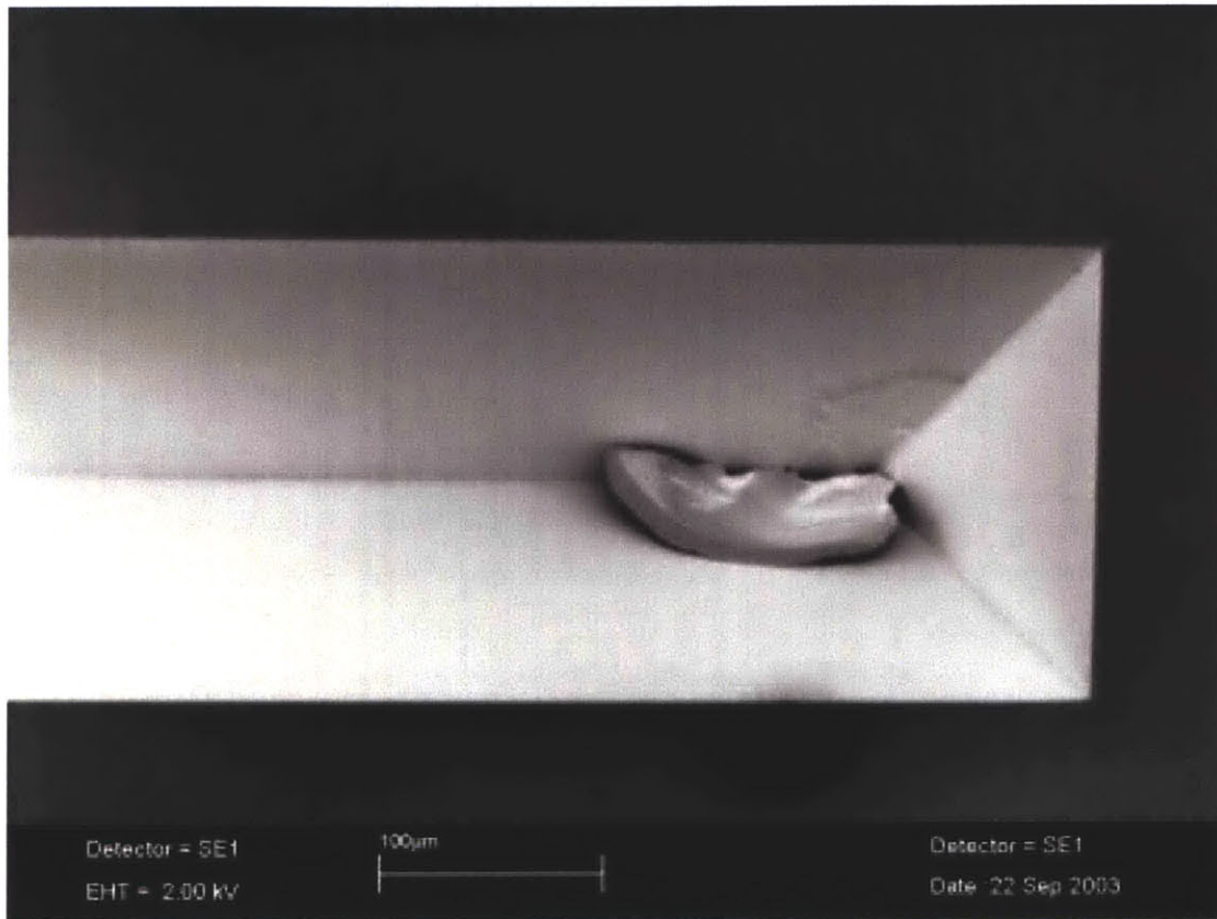
Figure 4-6: SEM image of the edge of a KOH-etched trench without gold.
