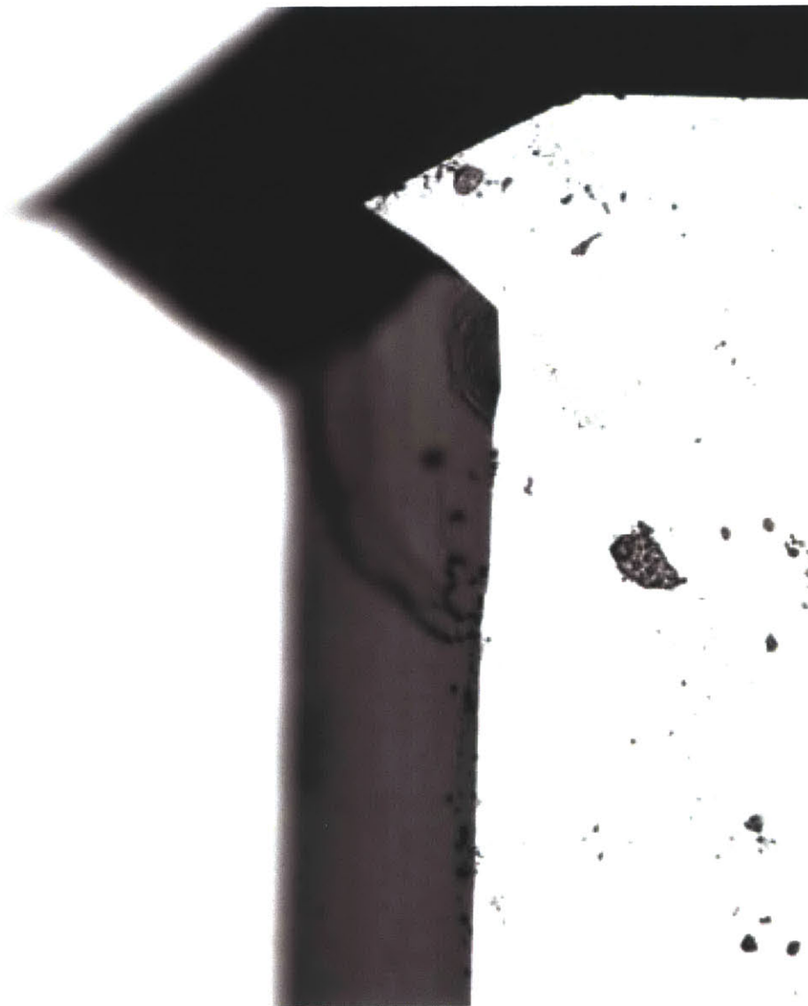
Figure 4-4: Microscope photograph of KOH-etched convex corner after gold deposition.
