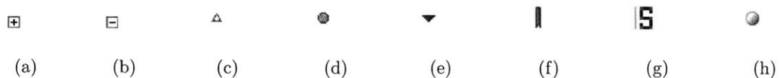
Figure 4-4: Icons used by the Outline view for StreamIt files: a plus box (a), a minus box (b), a state variable (c), a method (d), a filter (e), a pipeline (f), a split-join (g), and a feedback-loop (h).
