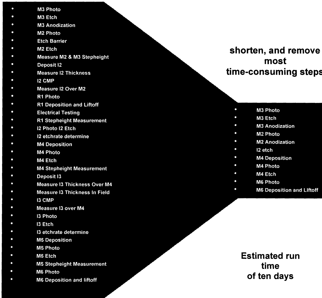
Fig. 2: Schematic chart of QC streamlining into TD process, illustrating removal of the most time-consuming steps and R1/M5/I3 layers.
