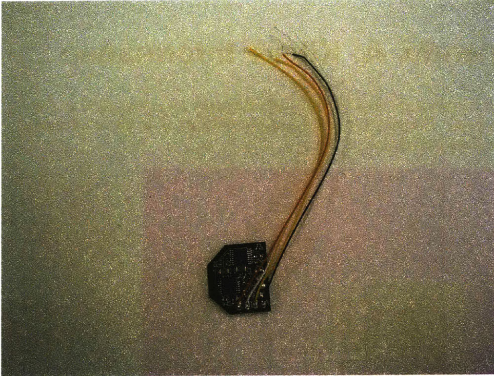
The custom logic board performs electronic signal translation between the reader and the mote, and also voltage regulation between the battery and the mote and reader.
