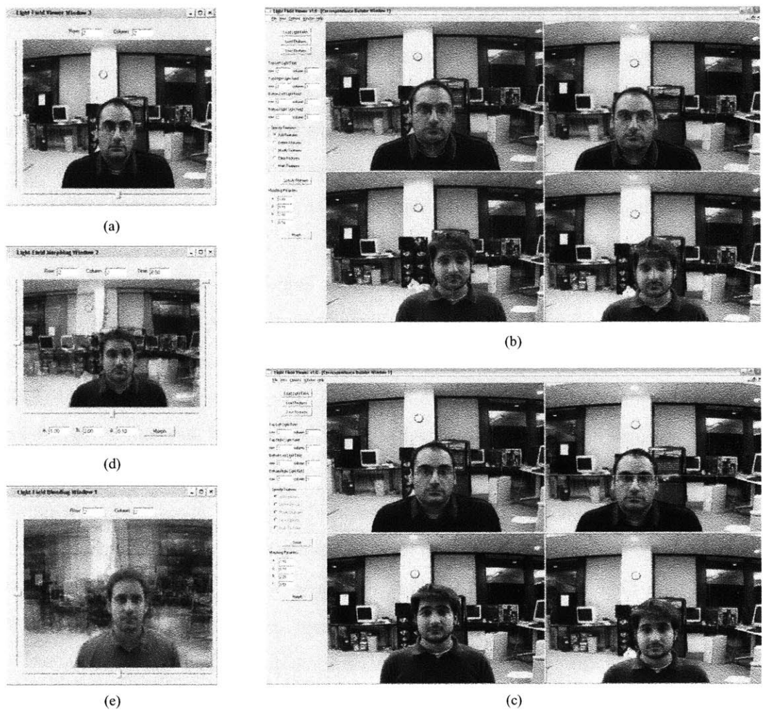
Figure 5-4: Light field morphing system: (a) light field viewer window, (b) correspondence builder window, (c) feature specification guided using epipolar line (in yellow), (d) morphing window with interpolated features overlaid, and (e) blending window with interpolated features overlaid.
