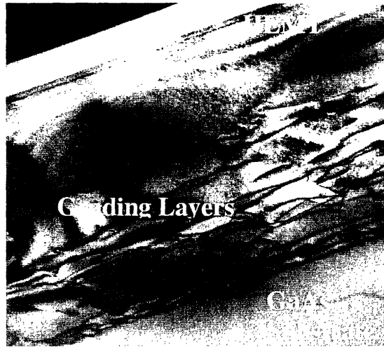
Figure 24: TEM cross-section micrograph of metamorphic HEMT material.
