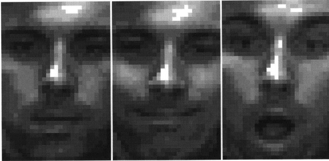
Figure 7-11: 2-D Full-Face templates of neutral, smile and surprise expressions used for tracking facial expressions. See Figure 7-14 and Figure 7-15(a).
