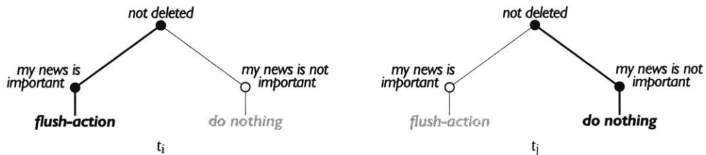
Figure 3.5. A schematic diagram that shows how a headline agent selects an action at two different situations at t_i and t_j .
