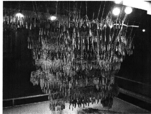
Figure 8: Catenary hanging model
