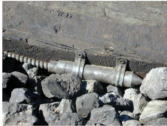
Figure 6.14: P5 clipped on the rail tie.
