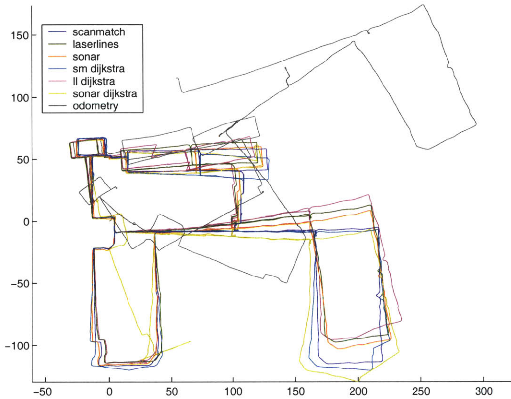
Figure 7-1: A comparison among the robot pose trajectories of the Killian Court data with different implementations and projections.
