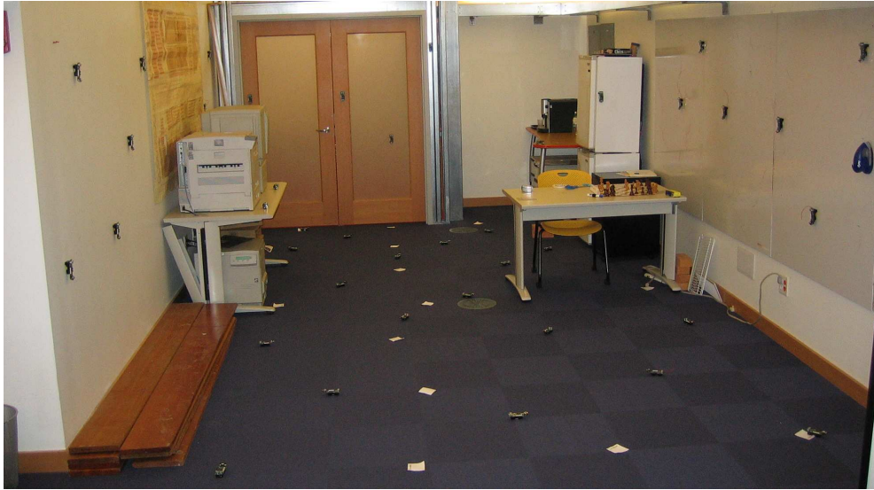
Figure 6: Environment used for initial 3d localization experiments. LaSLAT localized sensors to within 7 cm.
