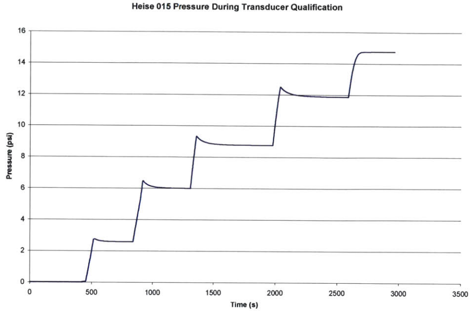
Figure C.1: Pressure history of Heise 015 during transducer qualification
