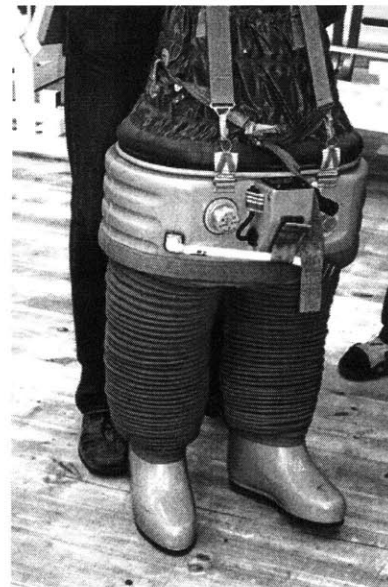
Figure 4. (a) Penguin suit and (b) Tchibis suit (lower body negative pressure), in its inactivated state (atmospheric pressure).
