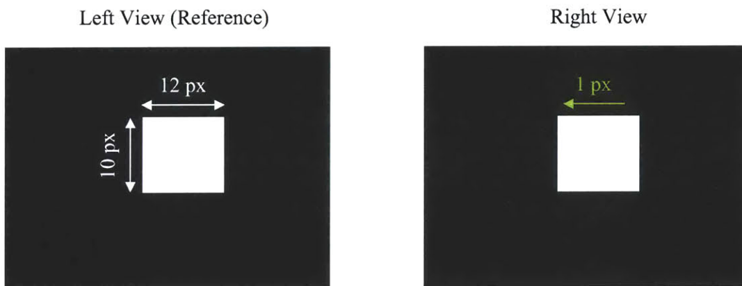
Figure 4-7: Static cue example. A white block of size 12 \times 10 pixel is shift to the left by 1 pixel .
