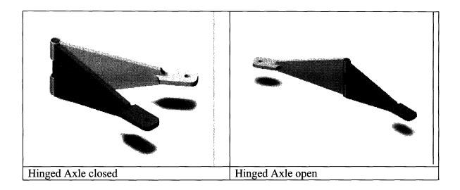
And additional potential benefit of the hinge is the ease involved in installing a locking mechanism. A simple deadbolt could lock the axle into the open position, making the power path even more rigid.
