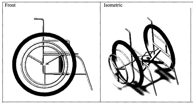
The DHRM weighs approximately two pounds more than the standard Whirlwind model wheelchair. It adds an additional inch of width to the overall chair, but this is still reasonable for most doorways.
