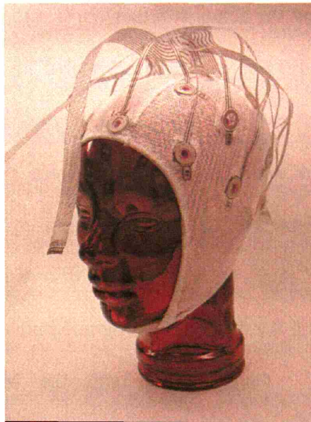
Figure 3.19. EEG cap featuring conductive ink-based electrodes and integrated motion sensors.
