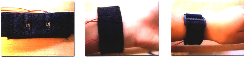
Figure 27: PSS wrist strap design. (Left) Sensor encasement. (Middle) Sensor-side of strap positioned on lower inside wrist over veins. (Right) Velcro and buckle side of wrist strap.
