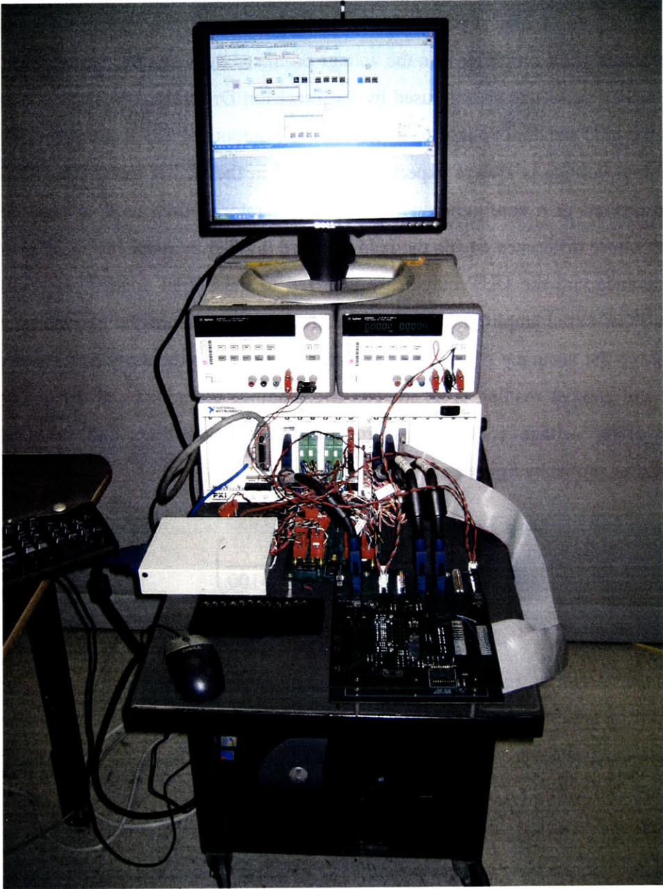
Figure 10. The assembled instrumentation amplifier AutoBench system.
