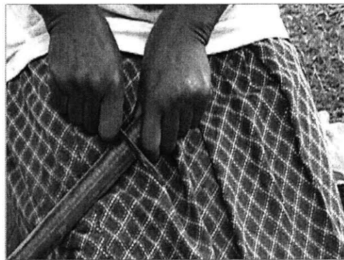
Figure 7-2. Oriang potter cutting PVC pipe to proper length with a hacksaw blade. (Source: Pihulic, 2005a)
