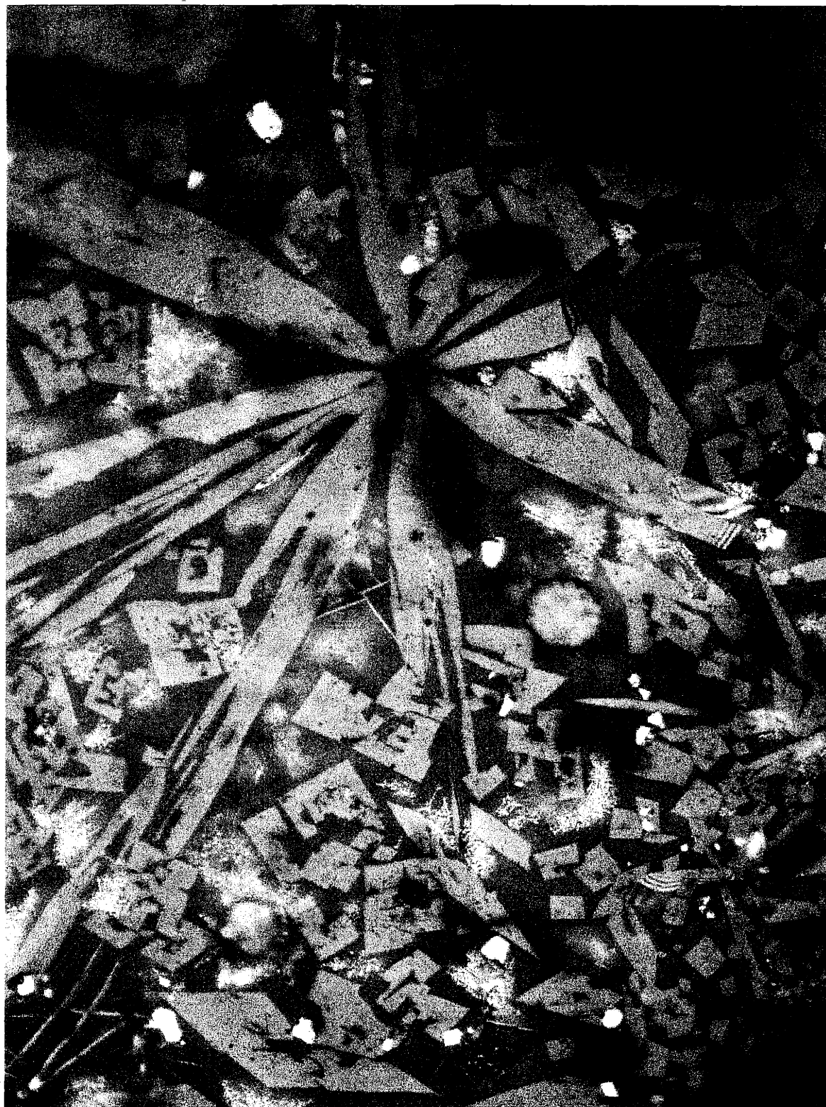
Figure 5.52 Matrix phases for MIT No. 241 \delta Zone 4, taken at a magnification of 500 (Matrix for MIT No. 241 \delta can also be seen in Figures 5.48b, 5.50, and 5.51)
