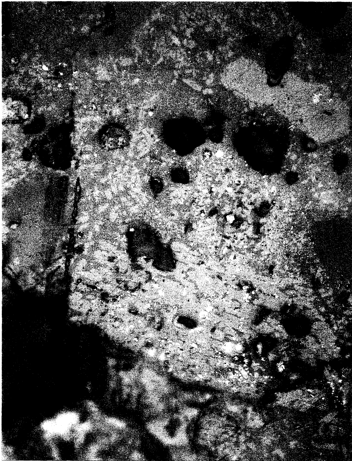
Figure 5.48a. Copper prills found in MIT No. 241 \beta at a magnification of 500, Zone 3.
