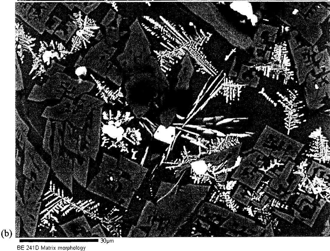
Figure 5.50. Dendrites in MIT No. 2418 Zone 4 (a) photomicrograph at a magnification of 500; and (b) SEM image with scale bar indicated.
