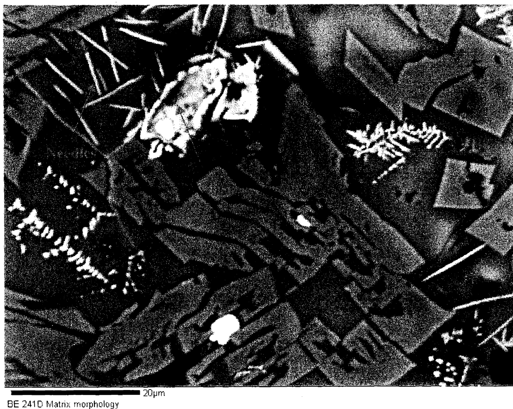
Figure 5.51. Clast and needle phases in MIT No. 241δ. SEM image with scale bar shown.
