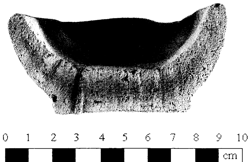
Figure 5.3b. MIT No. 5277: Section of modern crucible replica; Carbon coring provides proof that this replica was fired at a low (below 600°C) temperature when constructed.
