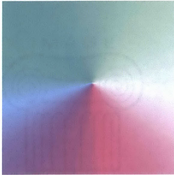
Figure 5-4: Bicolor absorption filter: Cyan and Magenta, blended together and graded from a transparent background
