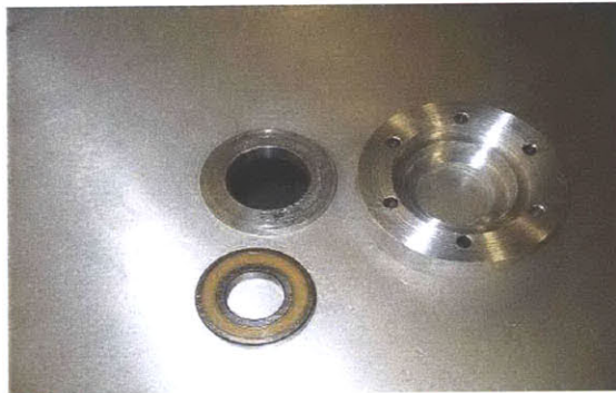
(a) Disassembled: Main bearings and casing.
