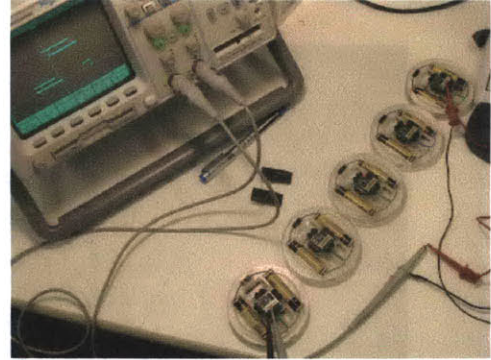
Figure 5-12: Topologies for various network diameters d used in this work. The oscilloscope probes are connected at the edge nodes of the network. The case for d = 4 is shown in the right figure.
