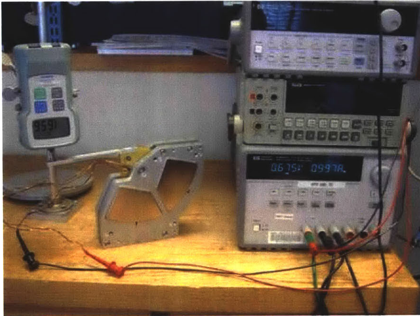
Figure 4-9. Set-up for initial force calibration on a single actuator.
