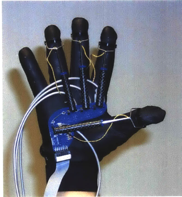
Figure 3-3. The second generation Rutgers Master is a body-grounded force-feedback device that uses pneumatic actuators to exert force at the fingertips. ( http://www.caip.rutgers.edu/vrlab/projects/rm2/system.html )
