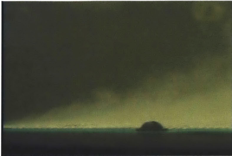
Figure 4.3 - Photograph showing bubbles starting at the leading edge at 75Hz 160 amps and less than 0.1 m/s
