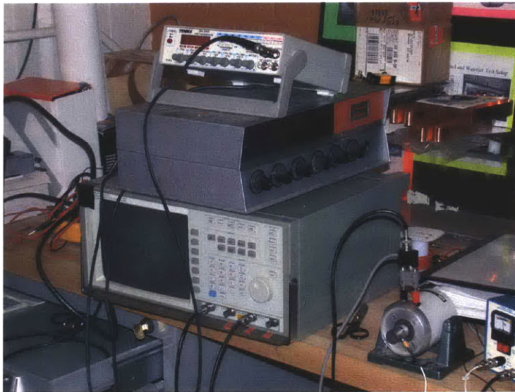
Figure 8.9 - Photograph showing mass shaker used on top of cassette for response measurements
