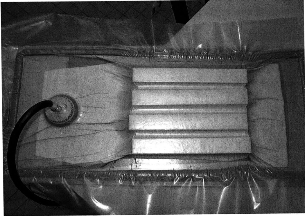
Figure 1: Vacuum Bagging Setup
